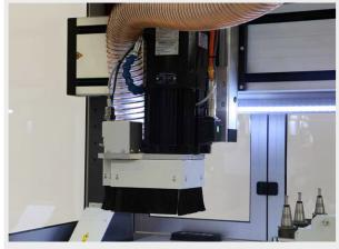
Option: suction device equipped with suction head
